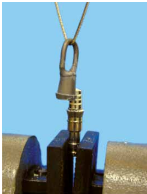
2 Retention test with testing machine.
