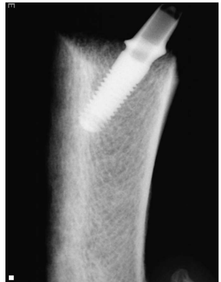
Fig. 1. X-ray of the 1P implant after inserted into the bovine bone. The implant is angulated to create 30 degrees in loading.
