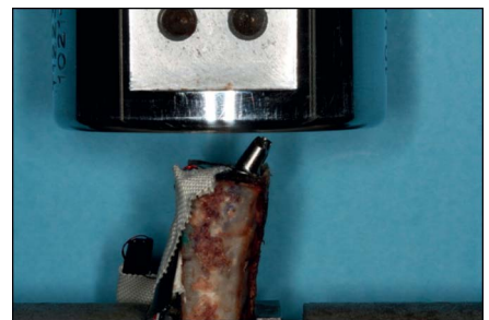
Fig. 3. The Instron loading machine creates vertical pressure on the abutment connected to the implant, resembling nonaxial loading.
